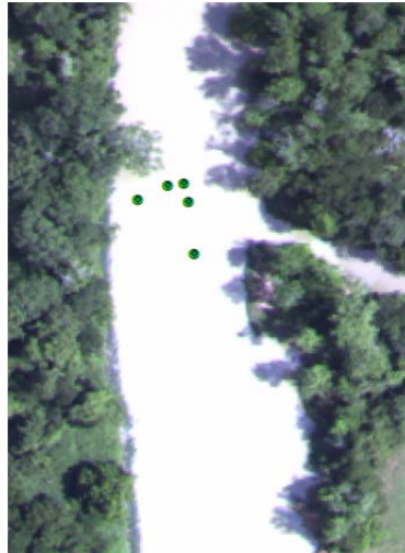
Figure 4.7 Auto gain issues at a sample point transect taken from June 23, 2010 imagery.
